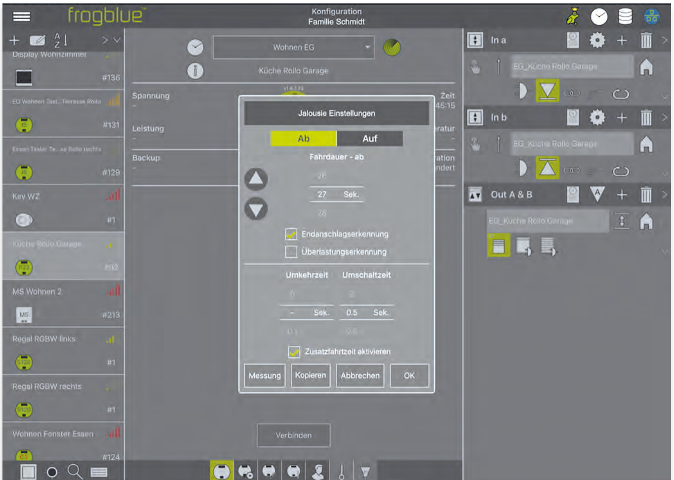
This ProjectApp section shows settings for blinds in a building equipped with over 200 frogs.
