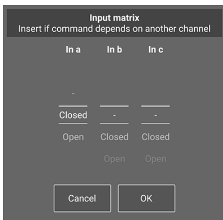
Figure: The settings in the input matrix if a status has been set for Input In a .
