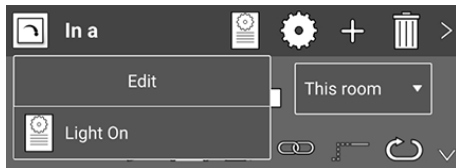
Figure: For the input In a , the Input macro Light On is available for selection.
