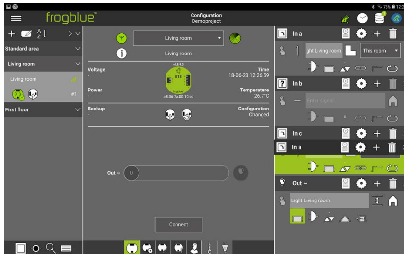
Figure: Input In c is marked light green and can be replaced.
