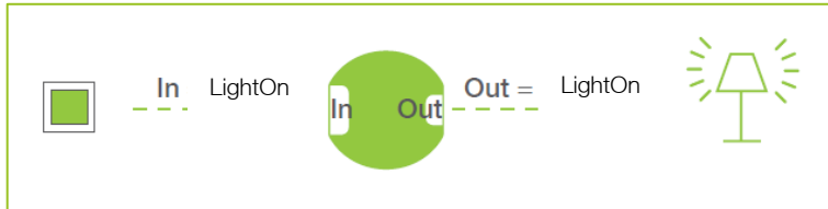
Figure: The Frog switches through when the text message in the input and output match.
