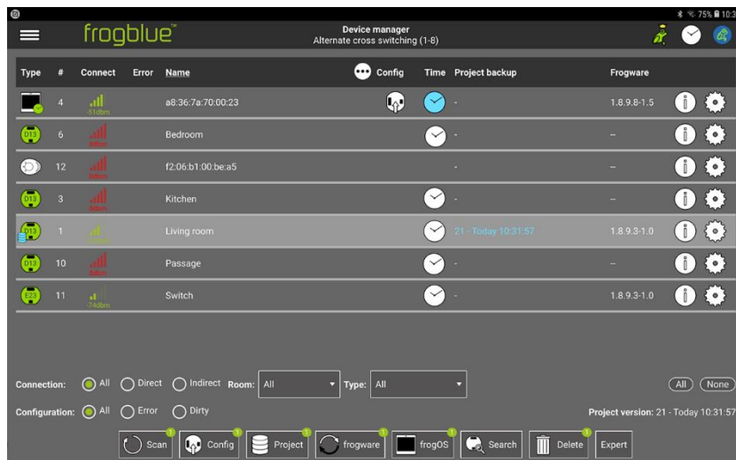
Figure: Green figures indicate possible actions for a Frog, frogKey or frogDisplay.
