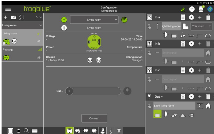
Figure: The message Light living room for the input In a and the output Out ~ .
